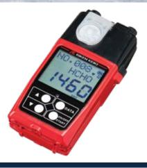
The FP-31 is a highly specific gas detector utilizing a proprietary colorimetric paper tablet to detect Formaldehyde. The instrument has a digital readout of the gas concentration on an LCD display. Readings are of average formaldehyde exposure over a selectable 15 minute or 30 minute period. This instrument does not respond to typical interference gases such as acetaldehyde, acetone, alcohols, ammonia, benzene, carbon monoxide, toluene or xylene.
