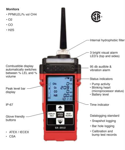
The GX-2012 is RKI's smallest personal 1-5 sensor gas monitor with a built in sample pump. Having 3 operating modes, the GX-2012 can be used for confined space, safety monitoring in it's Normal Operating mode; for leak investigation in Leak Check mode; and for underground leak checking in Bar Hole mode. When equipped with an optional TC sensor, the GX-2012 can measure 100% volume methane and dynamically auto range from % LEL to % volume. This is ideal for line purge testing.
