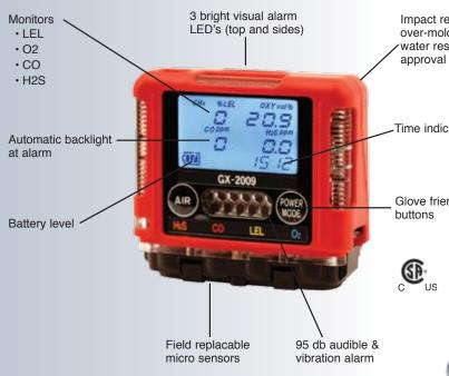
Impact resistant rubber over-mold body. Dust and water resistant with IP-67
