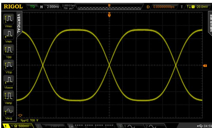
With rising and falling you have to be careful with these repeating square waves. Especially, it turns out at 20 MHz. A 20 MHz square wave takes 50 ns and the default trigger holdoff on the DS2000 is 100 ns so you are always catching one side of the wave because of the holdoff. If you really want to catch both
