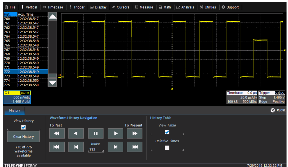
Figure 15: History Mode lets you scroll back in time to view acquired waveforms
