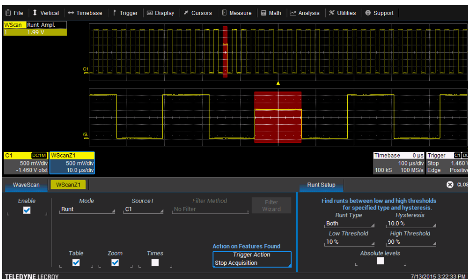
Figure 16: The WaveScan tool finds and automatically stops on signal anomalies
