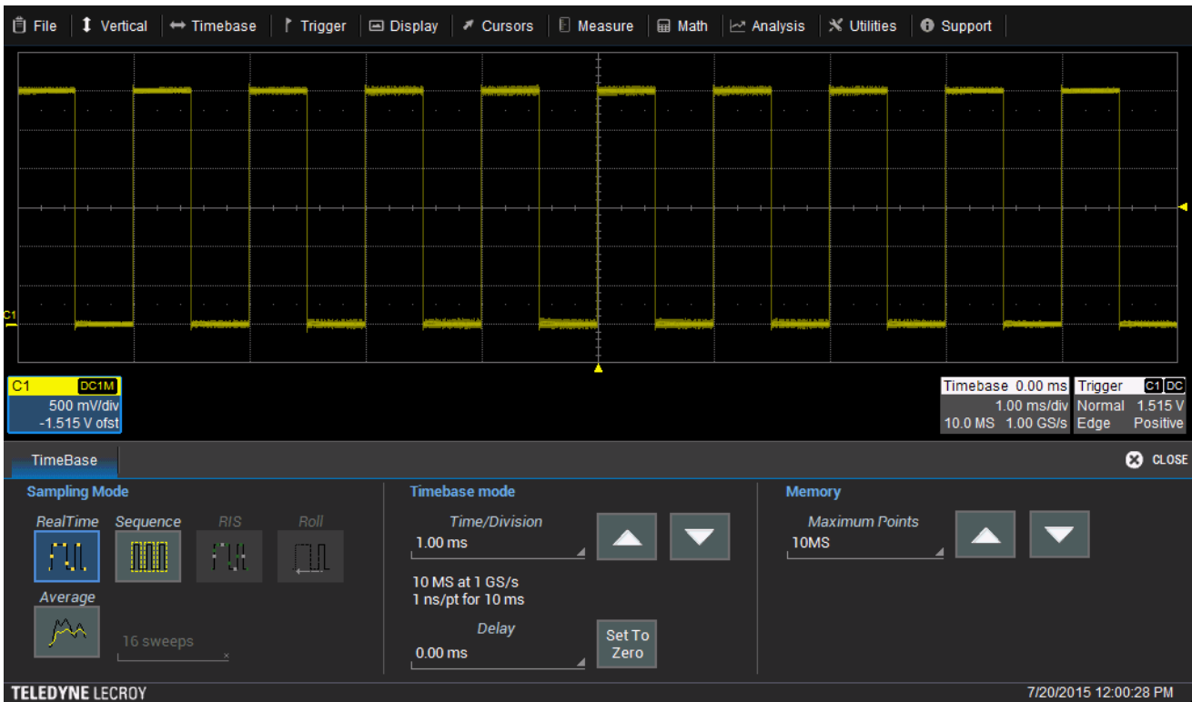
Figure 4: Touch the Timebase descriptor box to open the Timebase dialog
