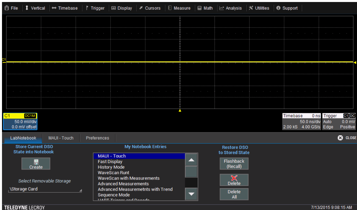
Figure 11: The LabNotebook dialog lets you recall stored setups and waveforms
