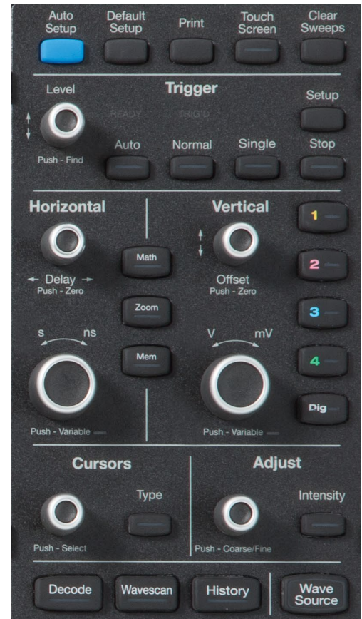
Figure 3: WaveSurfer 3000 front panel
