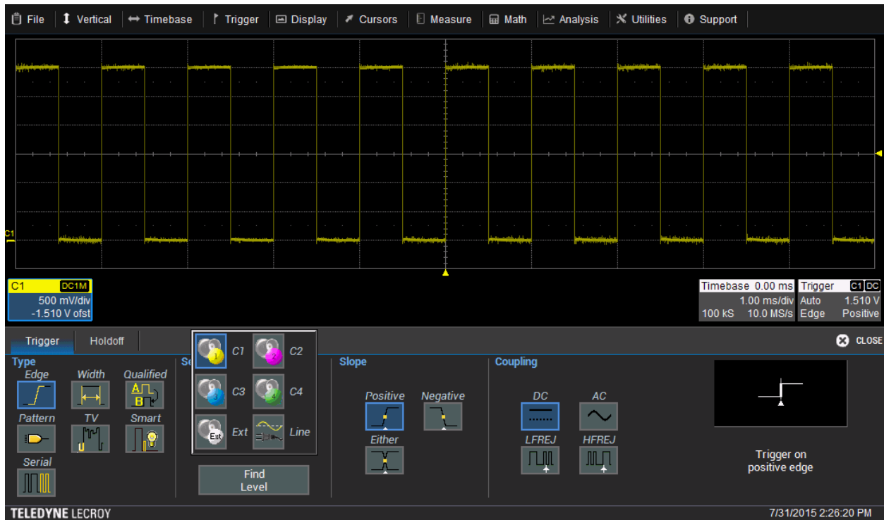
Figure 6: The Source field in the Trigger dialog box displays all possible trigger sources
