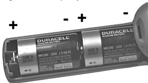
Figure 1. Properly Installed Alkaline Batteries
