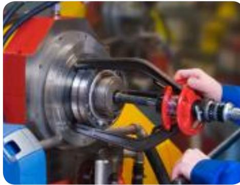
While every bearing has a pre-calculated service lifetime, research shows that not every bearing achieves it. When bearings fail to last for as long as they should, it is generally due to improper maintenance during key stages of the bearing life cycle. These can have a major impact on a bearing service lifetime, and include mounting, lubrication, alignment, basic condition monitoring and dismantling.
