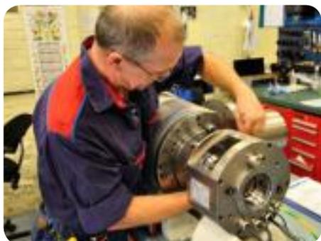
Keeping machine tool assets running in peak condition is vital to manufacturing operations. At the heart of this equipment is the spindle – so important to overall productivity, quality and efficiency that SKF has developed a specialized service programme just to manage this critical plant asset.
