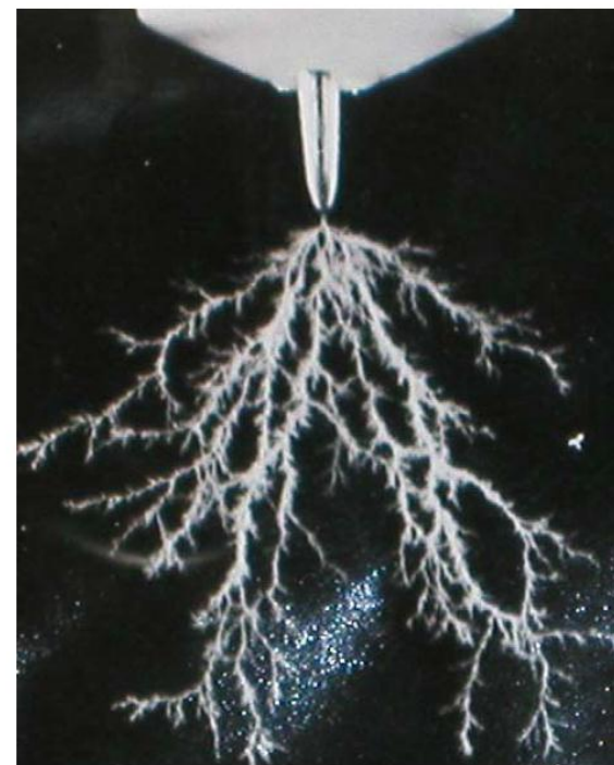
Treeing in Solid Insulation (Plexiglass)
