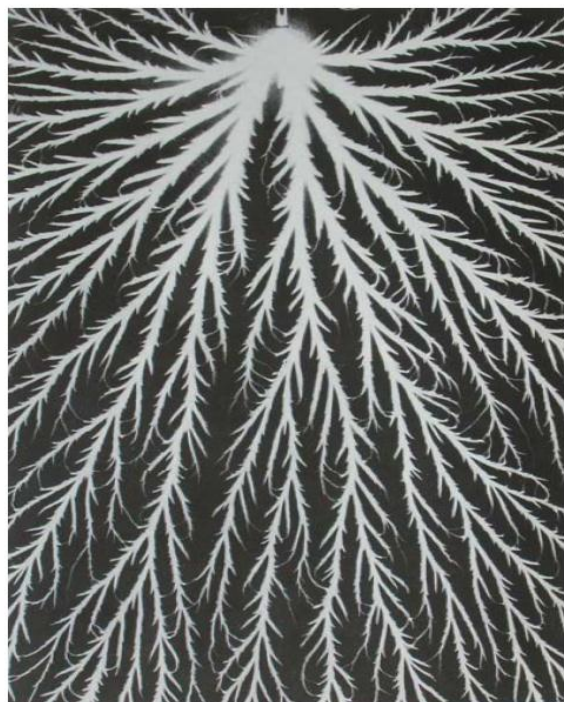
Insulation Tracking in Air
