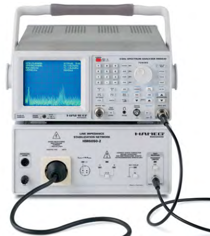
Measurement of conducted interferences via Spectrum Analyzer and LISN.
