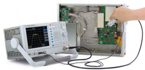
Determination of radiated distortion using a magnetic field probe (H-Field) and a Spectrum Analyser
