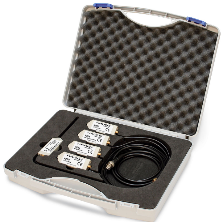
Fig. 1: Active H field sensors like this HZ540/550 set are near-field probes which can be used to measure the magnetic field strength. This magnetic field strength in the near-field is directly proportional to the conducted currents.
