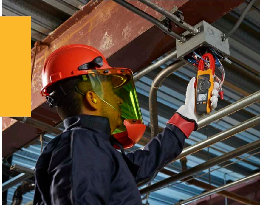
Choose a clamp meter rated to meet the electrical environment you'll be working in, as well as the resolution and accuracy of measurement you'll need for your testing.
