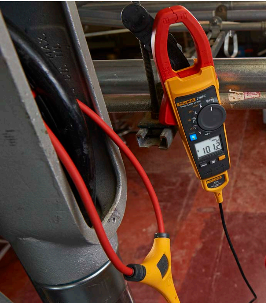
Use a flexible current probe for situations like this, where large conductors make it difficult to use the clamp meter jaws.
