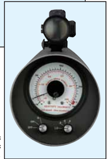
Needle swing shows differential temperatures instantly.
