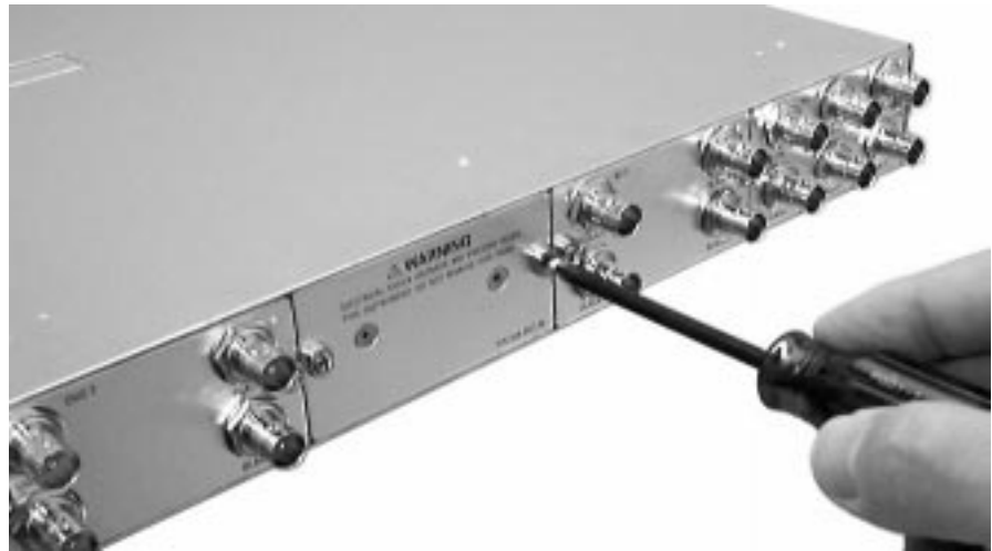
Figure 2-11: Removing the blank panel
