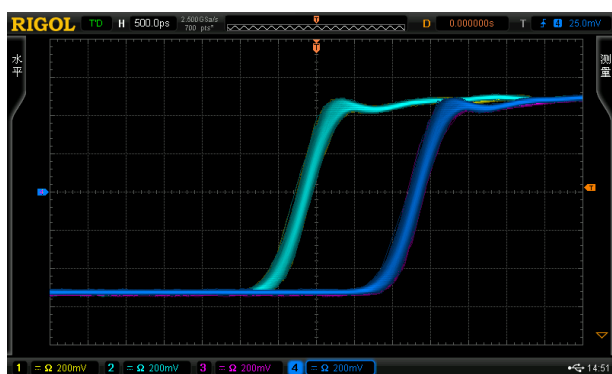
Figure 12 Failed Waveform of Delay Calibration
