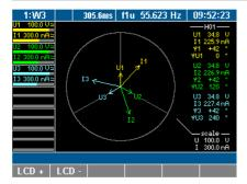
Vector display of HO1 up to 6 signals. For easy testing of the right connection of the instrument and quick overview of the phase angle of each signal.
