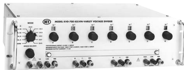
Figure 1.1. Model KVD-700 Kelvin-Varley Voltage Divider
