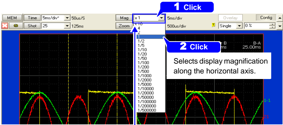
To view the whole waveform Click the [Mag] button to display the whole waveform.
