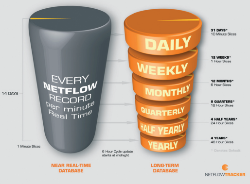
Figure 1 - NetFlow Tracker Flow Storage
