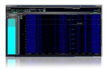
Spectrogram / Waterfall View for the identification of frequency hops, measurements of pulse rate, analysis of time variant spectra and the tuning of a VCO
