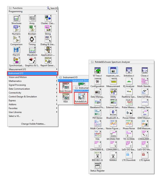
Fig. 2-4: Rohde & Schwarz Spectrum Analyzer driver in LabVIEW palette view under Instrument I/O -> Instrument Drivers -> Rohde & Schwarz Spectrum Analyzer.
