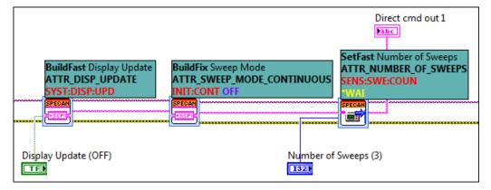
Fig. 4-15: SCPI command string building with two Fast Compose operations, and one Fast Write operation at the end.
