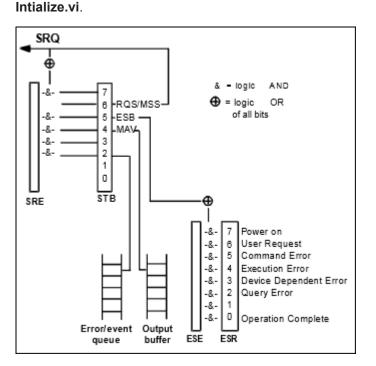
Fig. 6-2: Instrument status reporting system showing ESR, ESE and STB registers.
