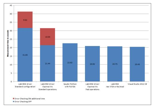
Fig. 5-2: HiSLIP duration time results of Measurement task.
