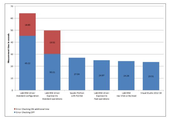
Fig. 5-1: VXI-11 duration time results of the Measurement task.
