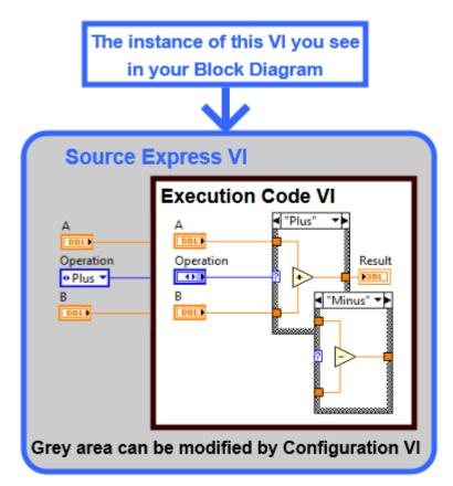
Fig. 4-1: Basic structure of Express VI. An instance of Express VI is visible in your code.
