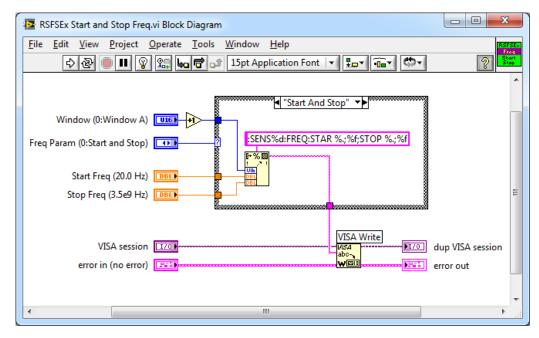
Fig. 2-1: Example of non-attribute based FSEx driver function VI.
