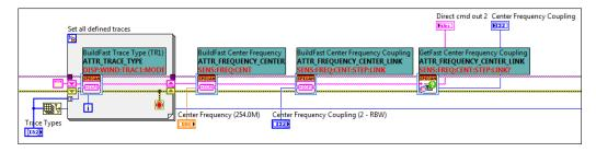
Fig. 4-17: SCPI command string building with several Fast Compose operations, and one Fast Read operation at the end, together with Error Checking.
