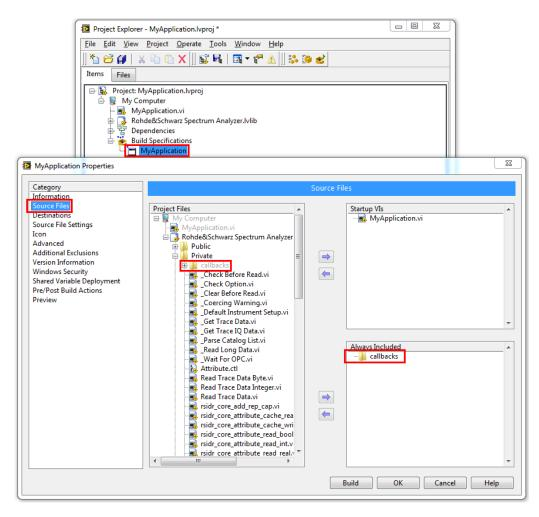
Fig. 6-1: Building an executable requires adding entire callbacks folder to Always Included set of VIs or folders.
