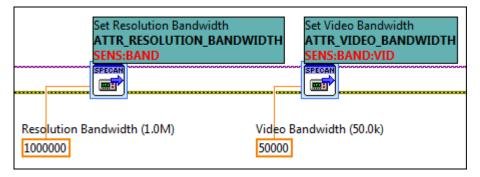
Fig. 4-16: Standard Write VIs that you can find in all driver functions.
