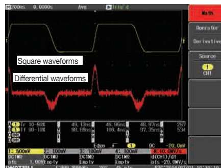
Differential calculation waveforms for square waveforms (rising 50ns, falling 100ns) (Displays the size of the time fluctuations (dv/dt) for square waveform edges.)
