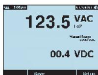
The feature also automatically displays the ac voltage of a live circuit, as well as any dc voltage, in a dual display presentation. Besides the everyday safety of reliable measurements, LoZ is also useful for monitoring residual dc voltage while troubleshooting electronic power controls such as those used for theatrical stage lighting or motor drives.
