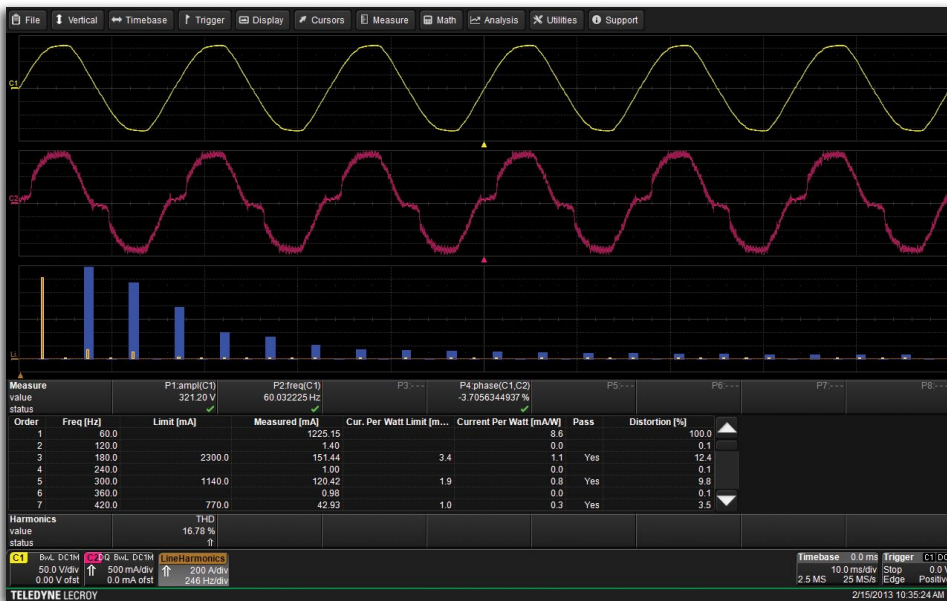
Both tabular and graphical displays provide conducted emissions for Class A, B, C, or D equipment as compared to standard templates of the EN 61000-3-2. The blue mask shows the test limits for compliance at each current harmonic.
