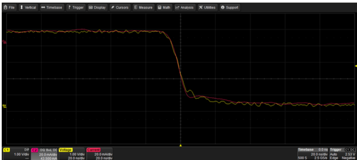
Falling edge of voltage and current traces after deskew adjustment.
