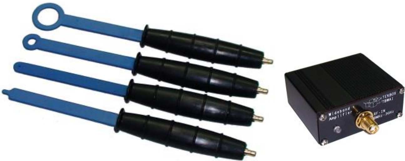
Picture 1 – from top, H20, H5, H10, E5; wideband amplifier
