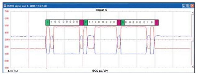
Figure 2. The data capture of the first three bytes of the Modbus RTU response at 500 µs/div. This representation includes a decoding of the response signal to clarify the slave node address, the function code and response data length in bytes (represented by the binary logic manually superimposed above the waveform).
