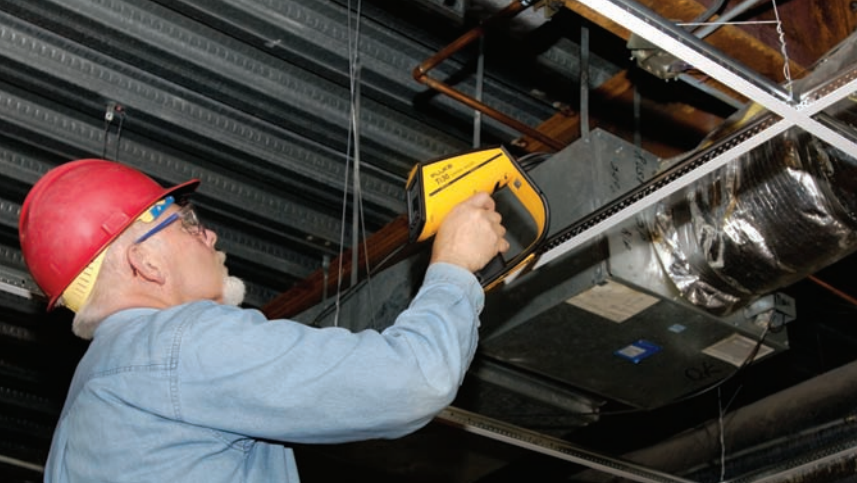
Figure 3. Figure 3: Qualitative measurements are fast for ducting, but accurate, quantitative measurements require compensating for reflectivity.
