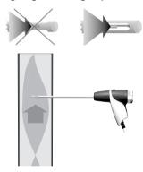
The thermocouple of the flue gas probe must not lie against the probe cage.
