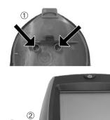
1 Remove sealing caps from the sides of the housing.
