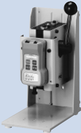
FGE-X with FGS-5S lever operated vertical test stand (sold separately)
