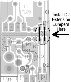
Take a moment now to check your previous solder joints for "opens" where the solder did not completely flow around the connection, or solder bridges between closely spaced pads. It seems the best time to identify these types of problems is now when you're focused on this section of the board, saving you time to try to retrace your steps later.
