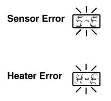
This error occurs when there is the possibility of a sensor failure (or a failure in the sensor circuit). **5-E** flashes and the power is shut down.
